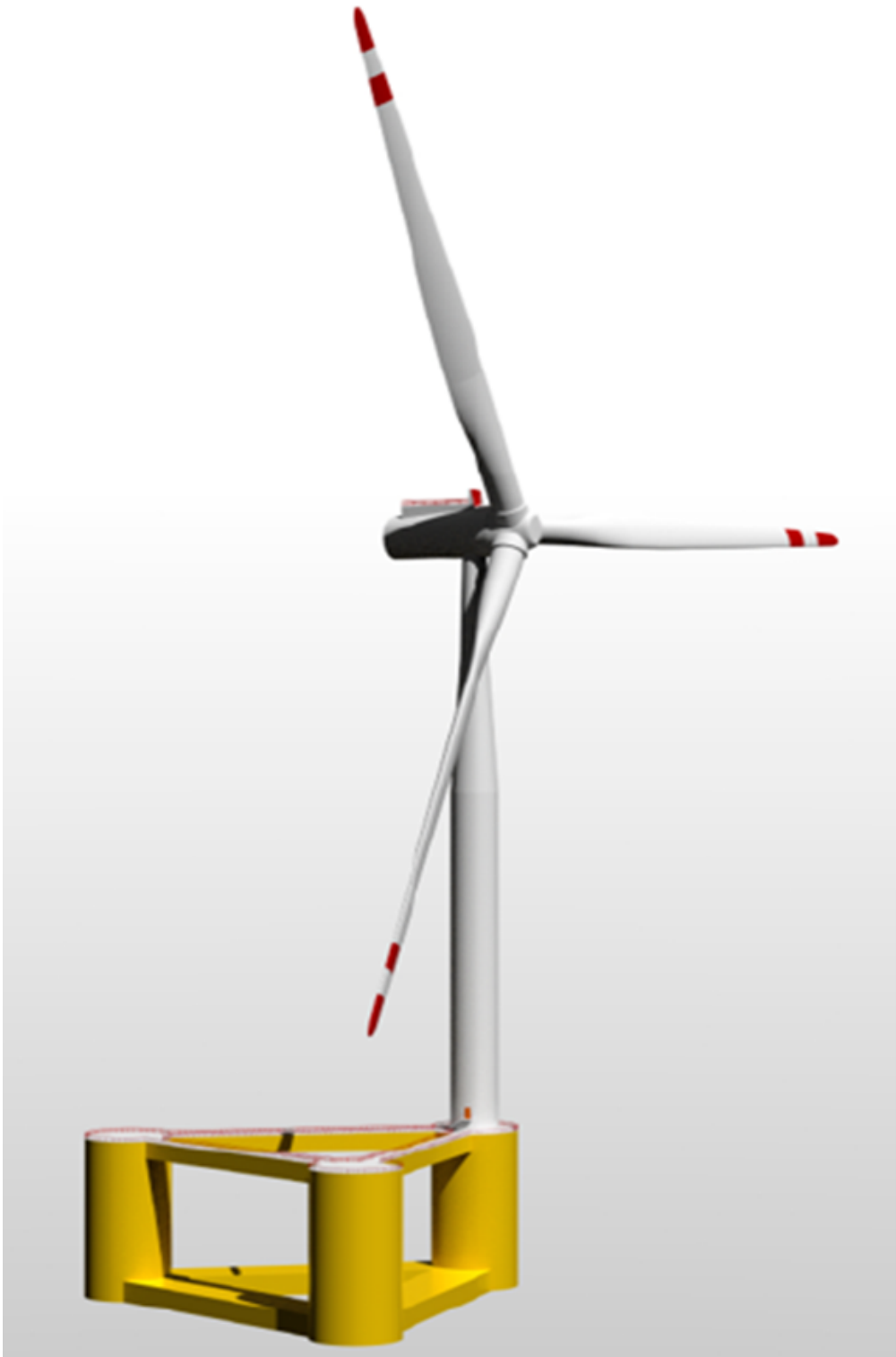
Figure 5.3: Full-scale model of INO WINDMOOR 12 MW wind turbine, obtained from [15].
