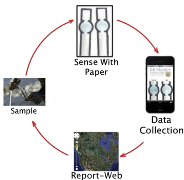
Figure 15. Concept of water quality evaluation using paper-based colorimetric sensors and a smartphone. Reprinted from Water Research, Vol. 70, Clemence Sicard, Chad Glen, Brandon Aubie, Dan Wallace, Sana Jahanshahi-Anbuhi, Kevin Pennings, Glen T. Daigger, Robert Pelton, John D. Brennan, Carlos D.M. Filipe, Tools for water quality monitoring and mapping using paper-based sensors and cell phones, Pages 360–369, Copyright (2015), with permission from Elsevier.
