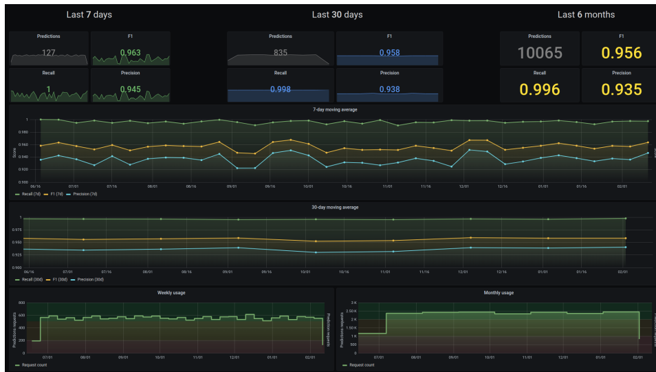
Figure 6.6: Illustration of performance monitoring of the machine learning models in real-time using Grafana Dashboard. See Appendix C for higher resolution.
