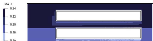
Fig. 10. Spatial simulation of yearly mean moisture content on untreated wooden façade.
