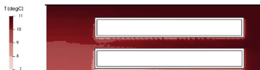
Fig. 9. Spatial simulation of yearly mean surface temperature on untreated wooden façade.
