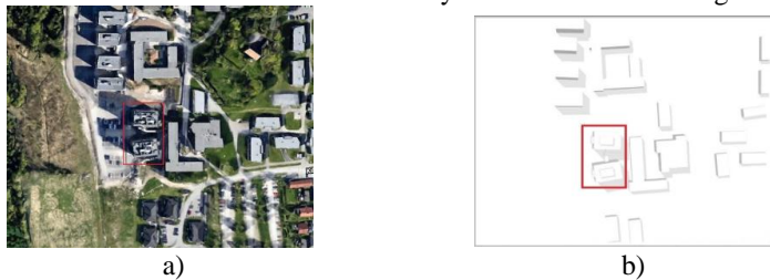
Figure 3. a) Satellite picture of the building complex and its surroundings, b) 3d model used for the CFD simulations. The twin buildings are marked inside the red frame.
