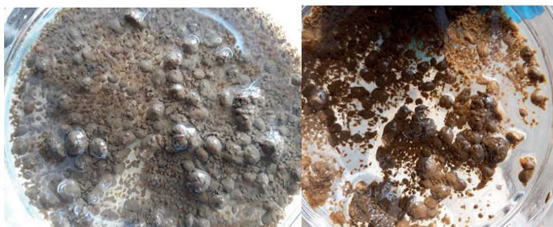
Figure 14. Active granules formed at the bottom of the first and second upflow sludge-blanket compartment of the ABR
