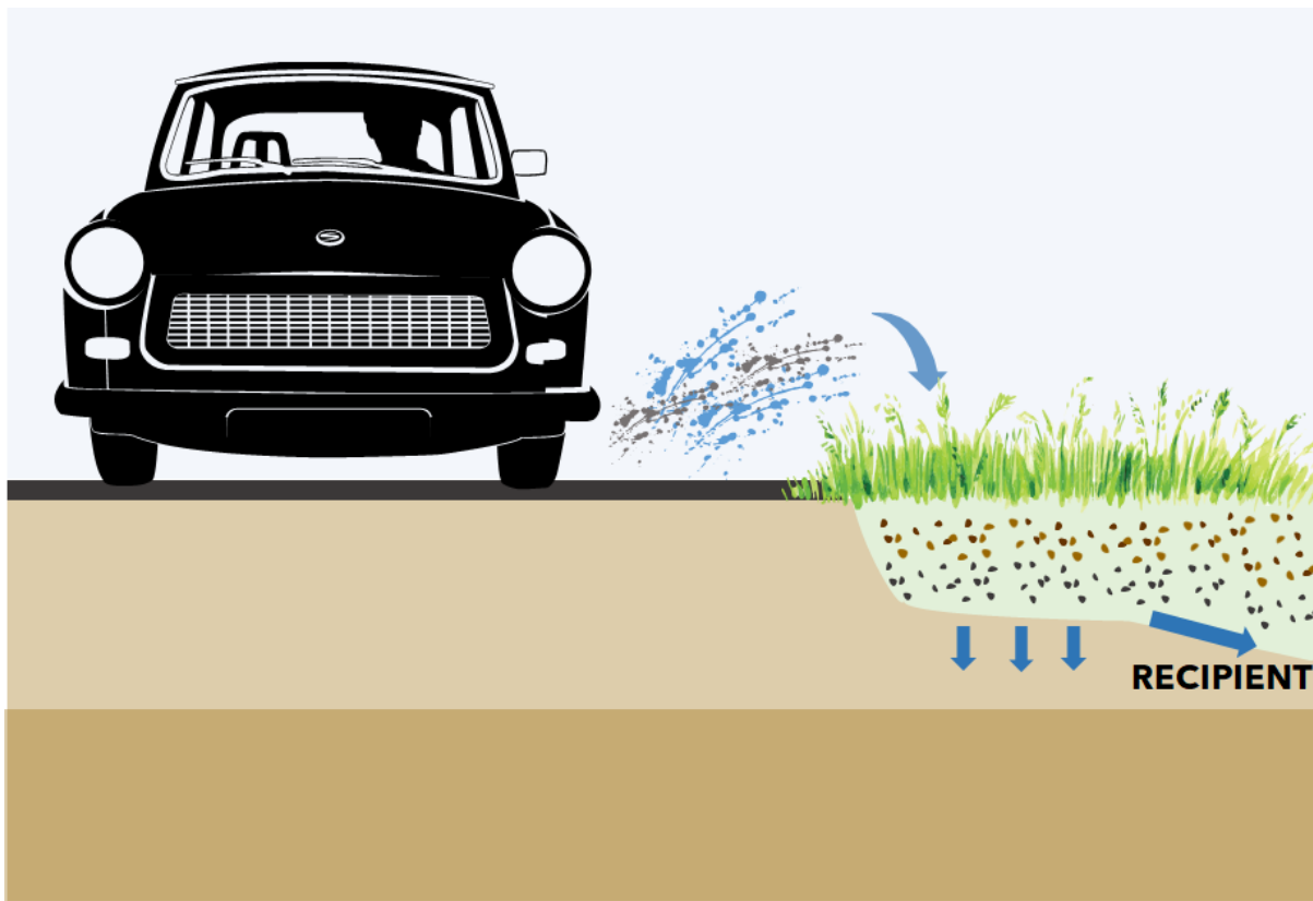
Figure 6. Conceptual illustration of a grass-filled swale (Illustration: E. Rødland, car and grass from freepik).
