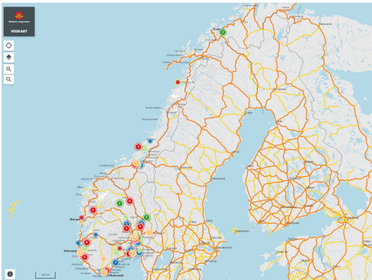
Figure 8. Overview of water treatment basins listed in the Norwegian road map application Vegkart ( www.vegkart.no ). Not all are shown on the map due to the scale. Markings: Water treatment basin (blue), Retention basin (yellow), Collection of pollution (red), Sedimentation (light green), Infiltration (dark green), Wetland (pink).
