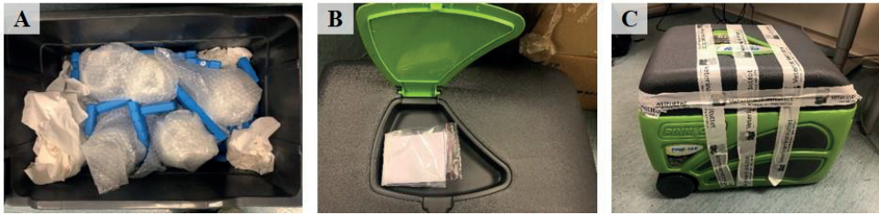
Figure 12. Transportation of water samples during the main field study. (A) For each sampled site, bottles were stored wrapped with bubble wrap insulation, surrounded by cooling elements in a 45 L Proxon cooler box (Pinnacle, Tokyo Plast International Ltd., India). (B) A filled out registration form ( Appendix ) was added to each shipment and (C) shipped together with the water samples to the laboratory of NVI (Oslo, Norway). Photo: L-V. Bernhardt.
