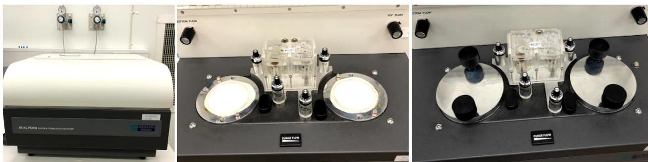
*Figure 6: OTR and CO<sub>2</sub>TR of PLA measured with Dualperm 8001 (photograph). Two samples of PLA were put in the analyser and adhered with grease (M&I, United Kingdom). From left to right: The Dualperm 8001 and two samples of coated PLA in the machine and the lids which covered the samples.*
