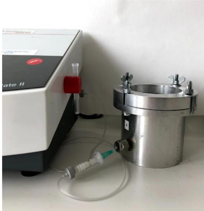
*Figure 8: Measurement of O<sub>2</sub>- and CO<sub>2</sub>- % in the gas cells with a headspace gas analyser (photograph). The O<sub>2</sub>- and CO<sub>2</sub>- % in the cells were measured using a Checkmate II (Dansensor, Denmark ).*
