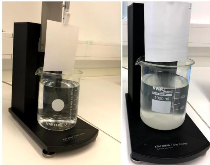
*Figure 13: Dip-coating of PLA and Invercote Duo in MMT-K10 and PEI (photograph). The substrates were immersed in PEI and MMT-K10 alternately. The MMT-K10 sank to the bottom quickly after stirring, which is seen as a white layer on the bottom (right picture).*
