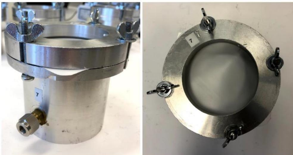
*Figure 7: The cells used for OTR and CO<sub>2</sub>TR-determination of PLA by using a method based on AOIR (photographs). The pictures show cells used to measure the OTR and CO<sub>2</sub>TR for PLA. Similar cells were used to measure air permeance of carton. The cells on the picture contains a sample of PLA.*
