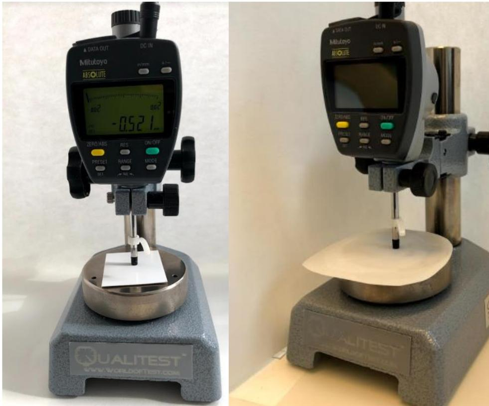
*Figure 2: Thickness measurements of the substrates (photograph) The thickness was measured using a Model 543 Film Thickness Gauge (Qualitest, Japan). The pictures show thickness measurements of uncoated Invercote Duo (left) and PLA coated with bentonite and PEI (right).*
