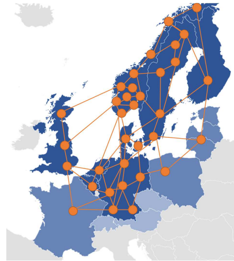
Fig. 1. Illustration of price areas and system boundaries in case study. Darker (blue) color indicates more detailed system representation.
