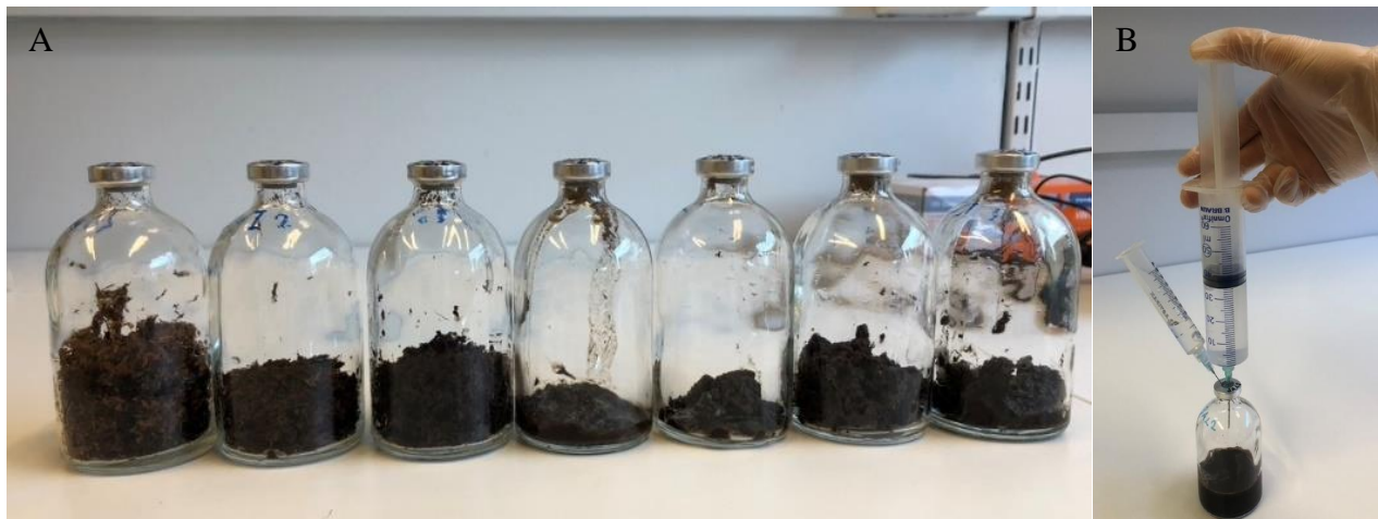
Figure 13: Photographs of loose and slurry treatments. A: A depth profile from Iskoras in serum bottles. From left to right: AL1, AL2, AL3, TZ, PF1, PF2, and PF3. B: Creating the slurry by adding ultra-distilled water through the septum with a syringe, while releasing overpressure through a syringe without plunger but filled with water to prevent air from entering the bottle
