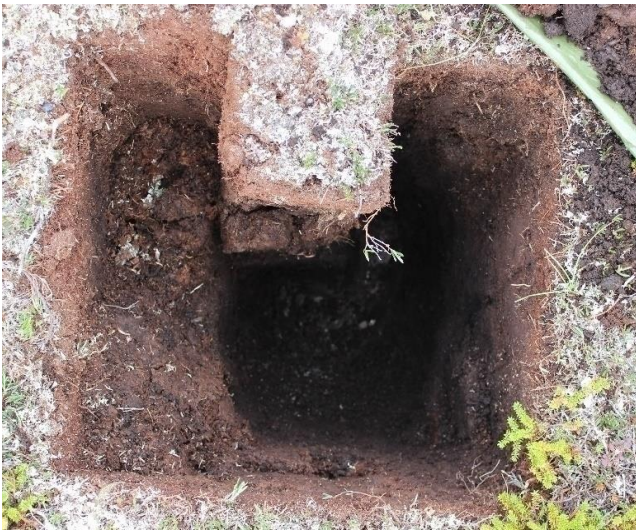
Figure 8: Photograph of sampling at Lakselv, showing how the AL was removed before taking the AL core
