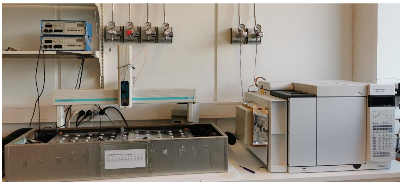
Figure 12: Photograph of the automated incubator used in the study; The unit consists of a temperature-controlled water bath with submersible stirring boards, a freely programmable autosampler periodically piecing the septum bottles with a hypodermic needle and a peristaltic pump transferring ~1ml headspace to a multi-channel gas chromatograph with loop injection
