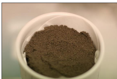
Picture 3: Amberlyst 15 catalyst before pretreatment in a sieve funnel covered with filter paper.
