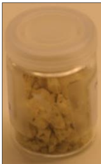
Picture 20: Melamine calcined at 400 C.
