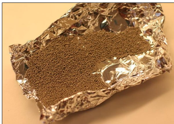
Picture 22: Amberlyst 15 wet ion exchange catalyst.
