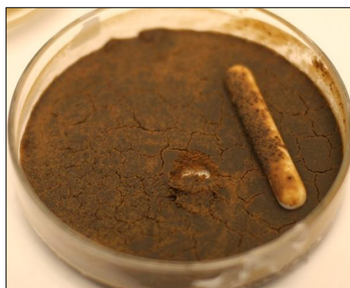
Picture 24: Recovered catalyst from the run with oleic acid and methanol. Some of the catalyst is fragmented.
