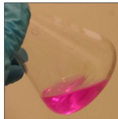
Picture 8: Sample after titration with color indicating basic solution.
