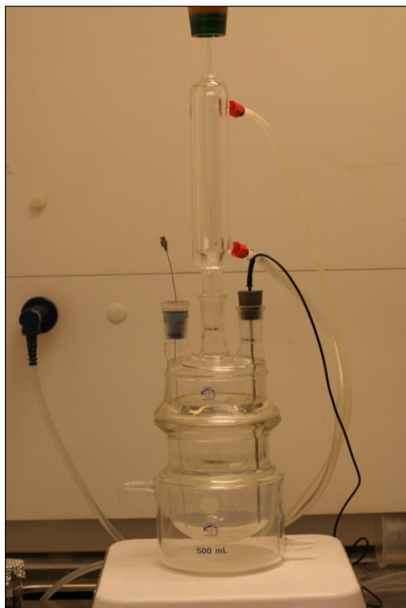
Picture 1: Glass reactor with accompanying accessories.
