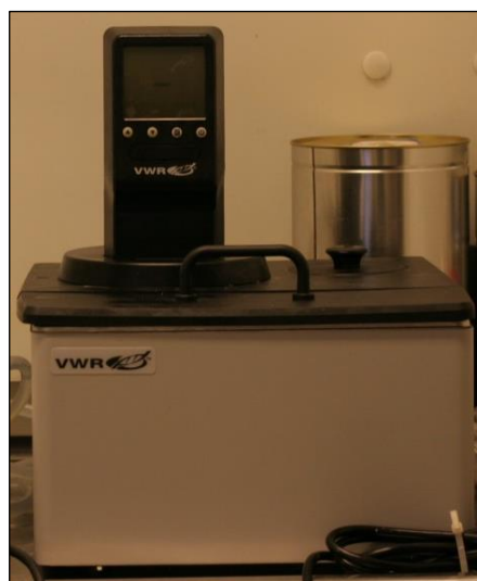
Picture 2: Warm water heater with circulatory pump.
