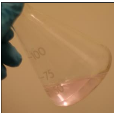
Picture 7: Sample after titration with color indicating neutral solution.
