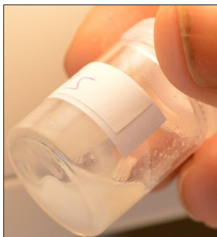
Picture 13: Sample of experiment with oleic acid, ethanol and melamine taken after 5 minutes of reaction time.
