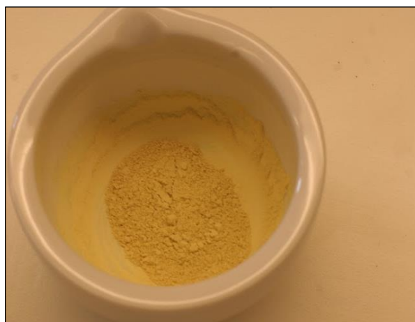
Picture 21: Calcined melamine crushed in a mortar.
