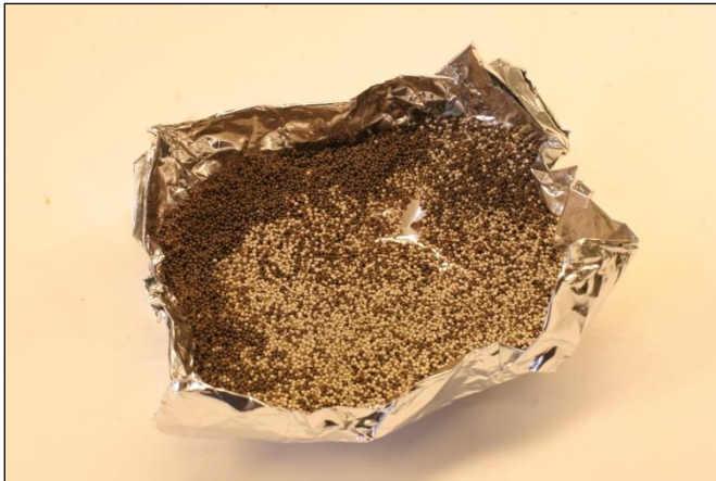
Picture 25: Amberlyst 15 wet ion exchange recovered from a run with oleic acid and ethanol at 60 C, 20% catalyst amount and 6:1 molar ratio.
