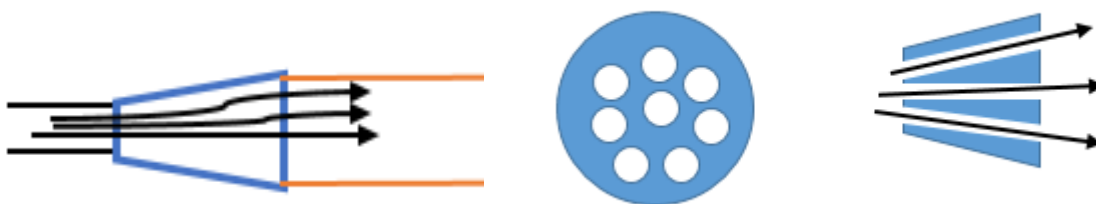
Figure 44: Simple sketches of two different solutions to overcome the turbulence. The sketch to the left is a cone-solution, chosen for this thesis. The sketch in the middle and the right demonstrates the flow separated by pipes to minimize the turbulence.
