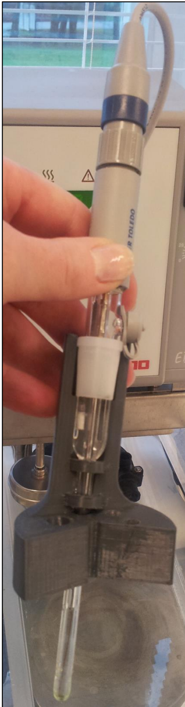
Figure 42: The titrator sensor placed in one of the parts of prototype 9 of the lid. Prototype 9 is similar to prototype 10, which is presented in Figure 40.
