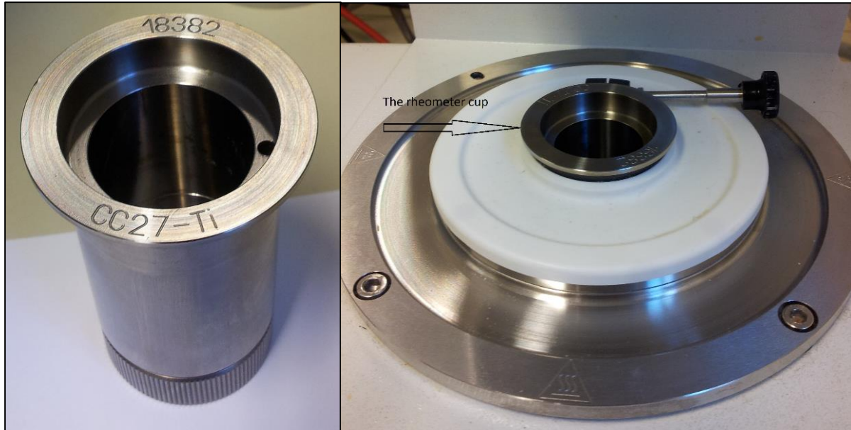
Figure 34: The rheometer cup used in this apparatus.
