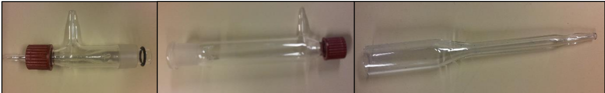
Figure 31: Left: Short outer buffer tube with inserted inner membrane-tube. Middle: Long outer buffer tube. Right: Inner membrane tube, there is two identical in the system.
