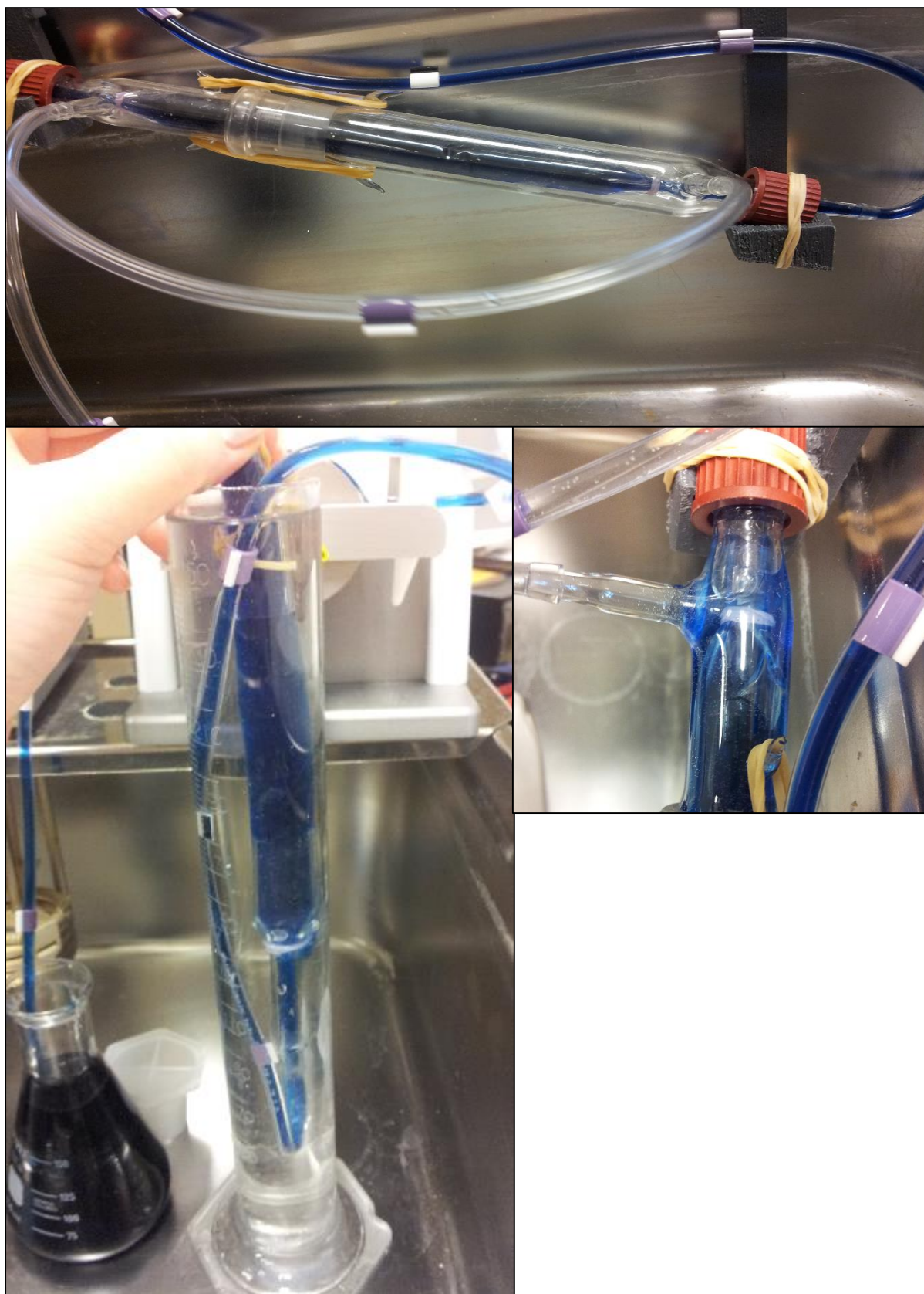
Figure 59: Above: The dynamic permeability test through the membrane where the colorant Evan's Blue was used. Bottom left: The static permeability test with Evan's Blue. Bottom right: Leakage after two hours of dynamic flow.
