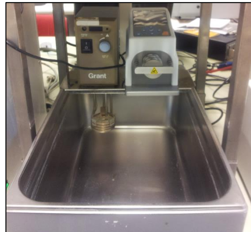
Figure 35: The heating container from Grant UK, used in this project. The peristaltic pump is placed beside the heating controller, saving room and volume of the entire apparatus.
