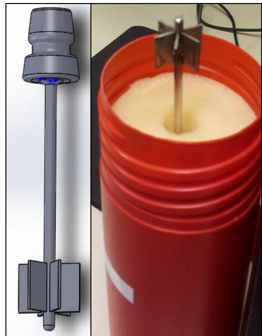
Figure 33: Left: The probe sketched in SW (scanned in a 3D-scanner). Right: The EMKA600 model in its container.
