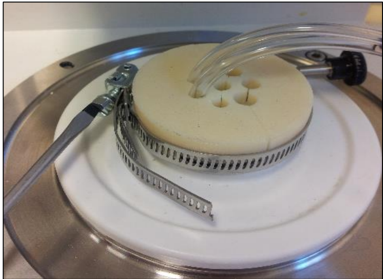
Figure 41: The hose clamp around the first printed prototype. A screwdriver with a flat head is used to tighten the hose clamp.
