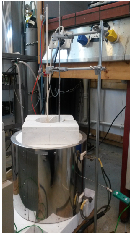
Figure 6: The furnace used for heating the salt, one can see the K-thermocouple in green to the bottom right, as well as the red S-thermocouple more in the back
