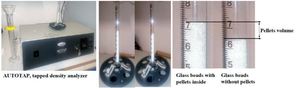
Figure 3.1 Demonstration for measuring the volume of feed pellets for specific density (SD) determination
