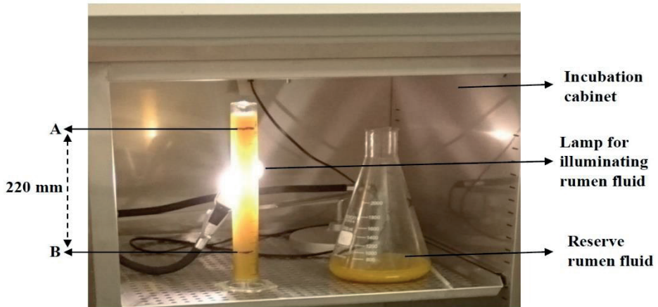
Figure 3.2 Apparatus for measuring sinking velocity (SV) of feed pellets
