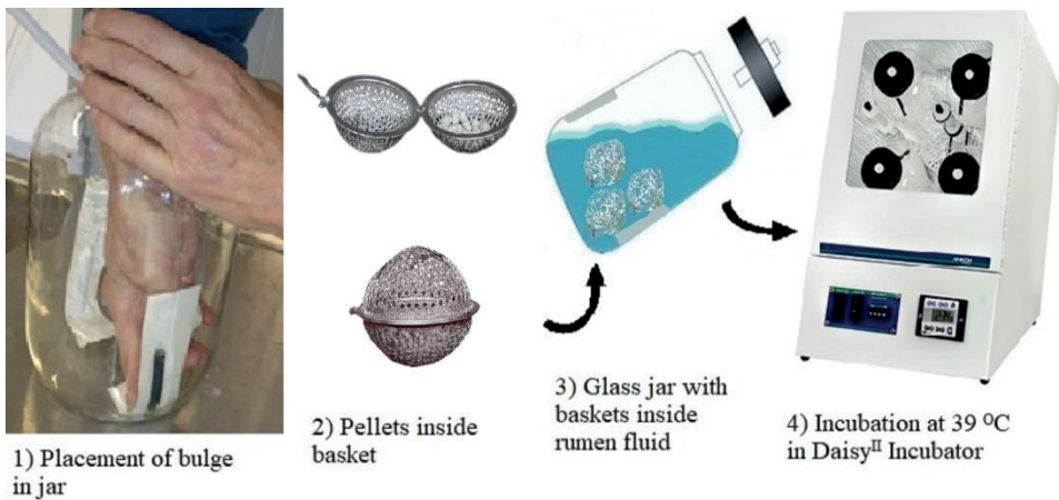
Figure 3.3 Demonstration of fluid stability index (FSI) test up to incubation. After incubation, baskets were placed in an oven at 103 °C for 18 hours for drying
