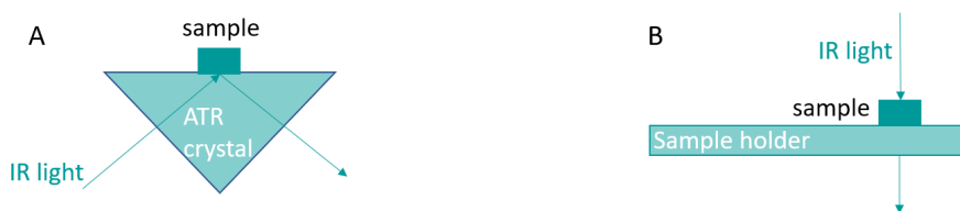
Figure 1.5: Schematics of FTIR measurement modes that were utilized in this thesis; A- Attenuated total reflection, B- transmission mode employing a high throughput system.
