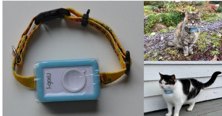
Figure 2: GPS unit i-gotU GT-120 with collar. To the right, unit is attached to study subjects; cats P331_9329079_Mie (top) and P331_9329674_Molte (bottom)
