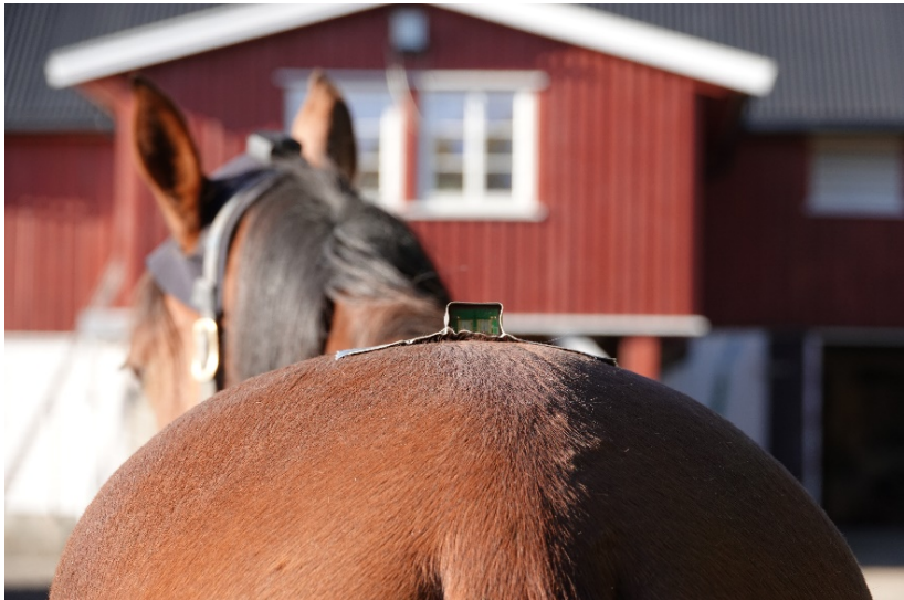
Figure 16. Correct placement of the pelvis sensor on the midline of the horse.
