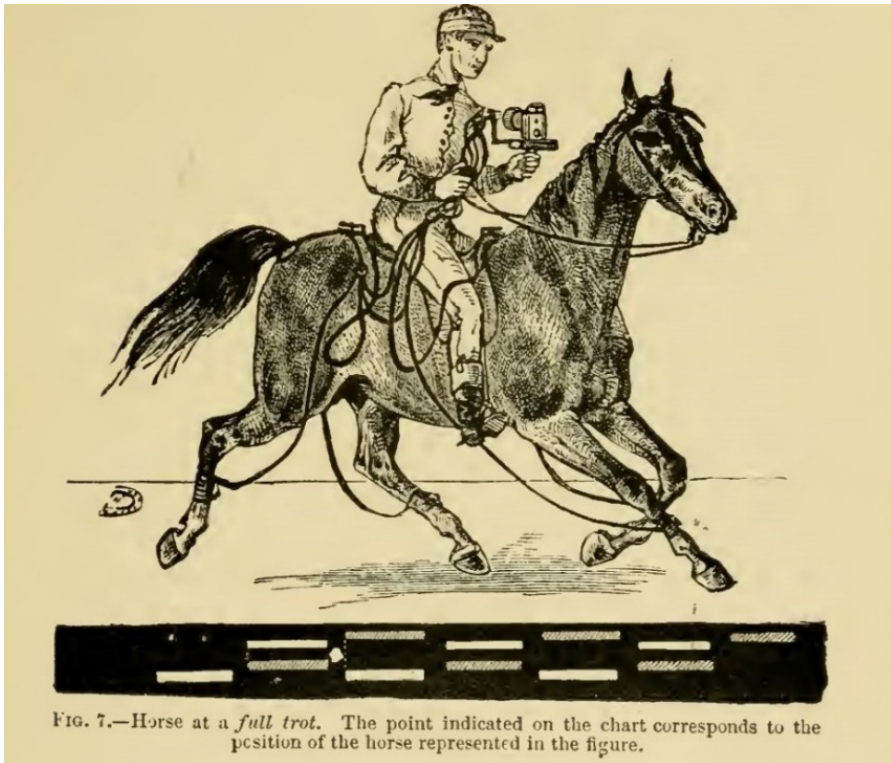
Figure 6. Illustration of Marey's pneumatic device to determine limb placement. Note the chart at the bottom of the image, showing the diagonal footfalls of the trot, and the point indicating that the horse is in a phase of suspension on the image. From Marey: Movement (1895). 157 Courtesy of the Biodiversity Heritage Library/Webster Family Library of Veterinary Medicine (copyright expired).
