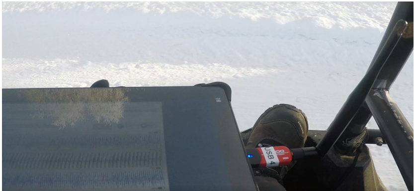
Figure 18b. Collecting data from the horse in 18a. Tablet running the system software; the USB Bluetooth antenna (red) is fitted with an enforcer/extended range antenna (black).
