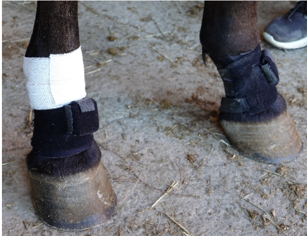
Figure 15. Pastern sensor wraps and additional tape. Only the right forelimb pastern wrap contains a sensor.
