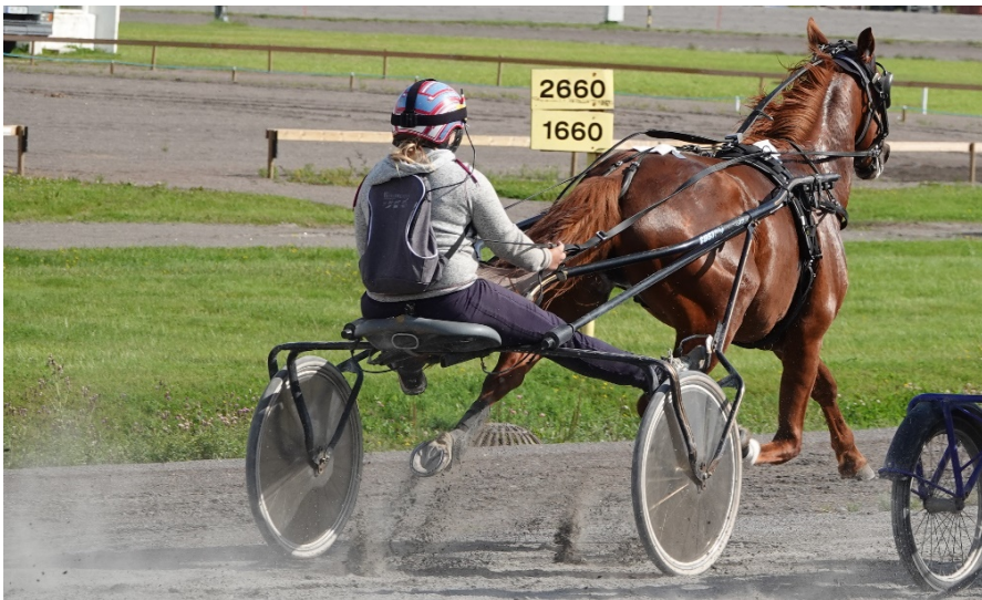
Figure 19. The driver carries a backpack with the tablet running the LL system software. To ensure continuous Bluetooth connection to the sensors, the Bluetooth antennae is taped to the driver's helmet and connected to the tablet via an extension cord.
