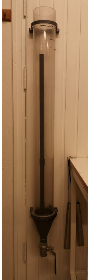
Figure 3.14: Tube used to measure Sinking Speed
