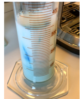
Step 4. Quickly pour the milk foam into the stained measuring cylinder in a tilted position, and then measure the volume (mL) of the foam.
