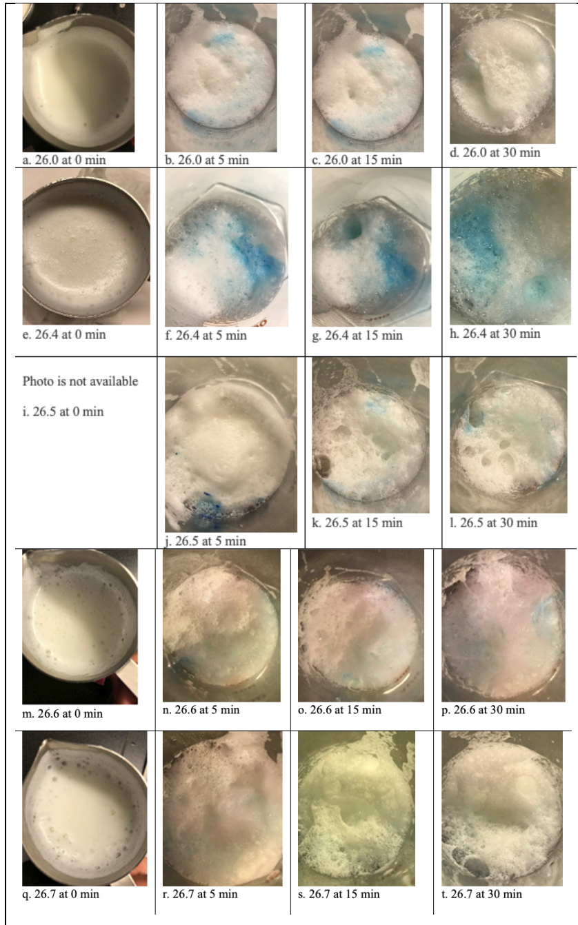
Figure 24. The foam appearance of standardized milk inoculated with Pseudomonas strain 26 from 0 – 30 min at Day 0, 4 & 5 (Trial 1).
