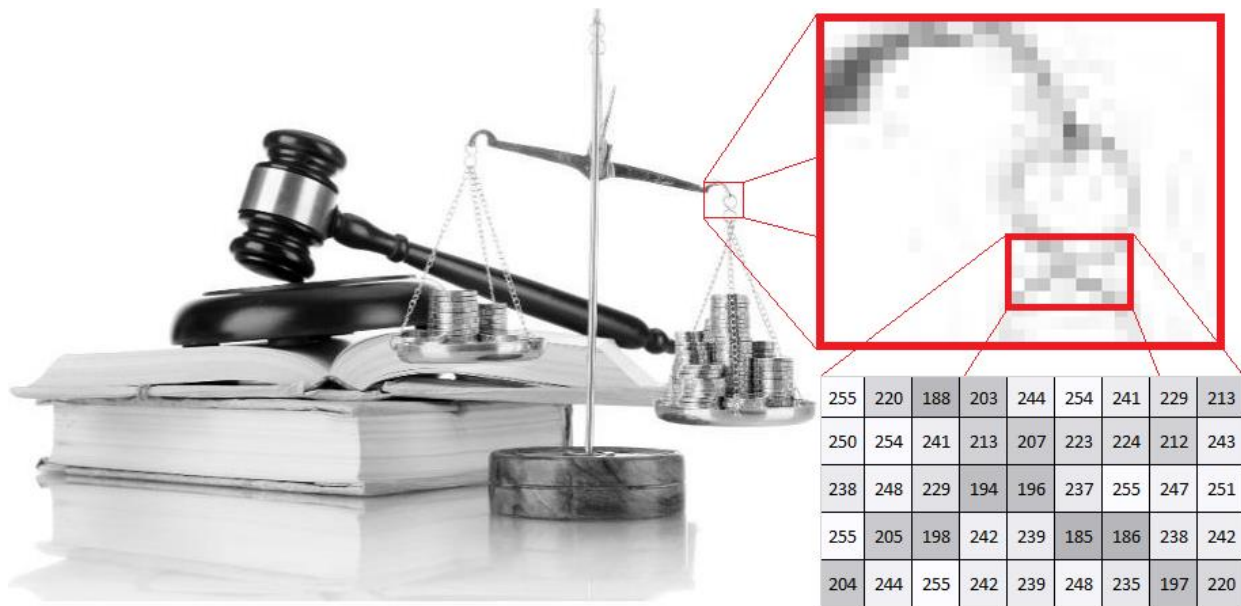
Figure 3: Illustration of how a grayscale image is composed of pixels; cells containing intensity values in a matrix. Image object (left) obtained using paid subscription from https://lucid.app/ .
