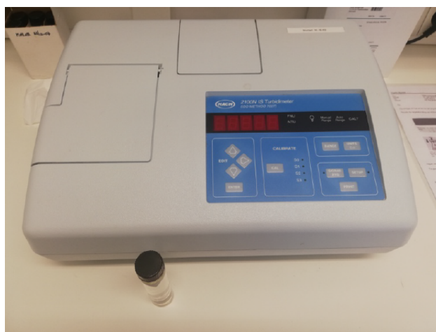
Figur A.1: Turbidimeter, Hack 2100N. (Teigset, 2019)
