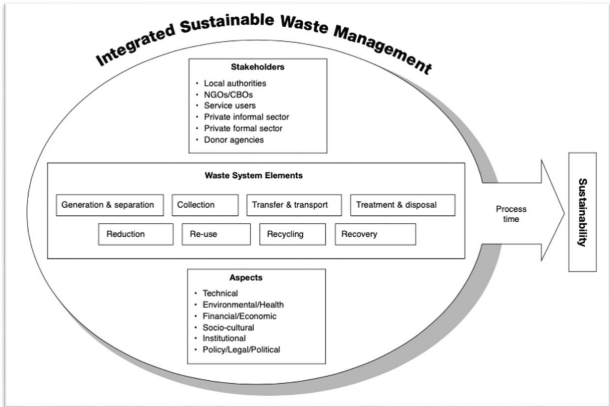
Figure 3: Integrated Sustainable Waste Management model (Anschütz et al., 2004).
