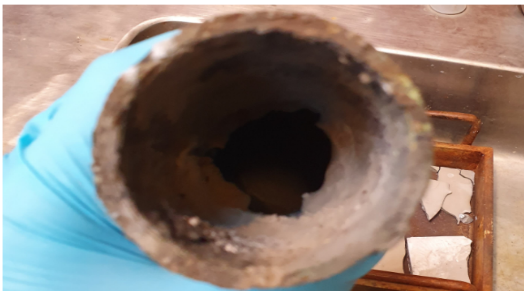
Figure 4.21: The figure shows a nickel crucible after being emptied of FLiNaK salt. There is solid MgO attached to the insides of the crucible, showing that much of the MgO has not been dissolved in the molten FLiNaK salt.
