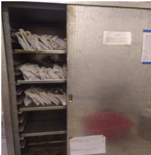
Fig. 12A: Samples dried in oven under 62 °C for dry weight. Picture: Ellen Kusi
