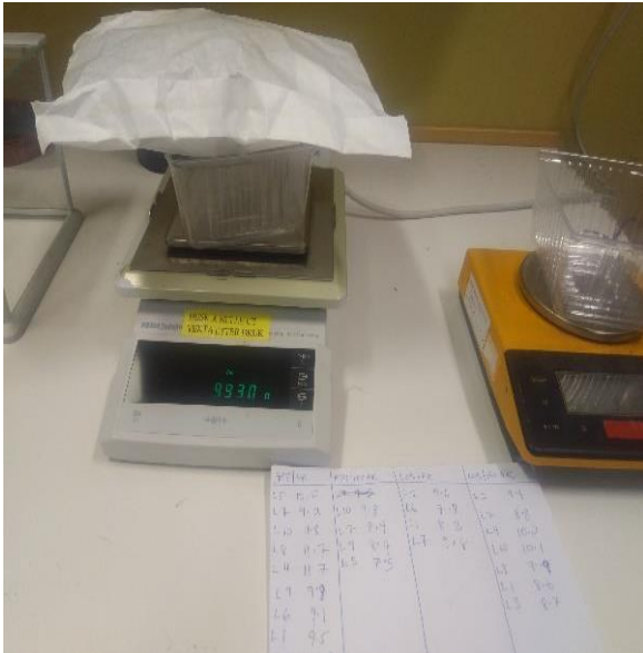
Fig. 11: Image showing how samples were weighed with accuracy of 0.01g. Picture: Ellen Kusi
