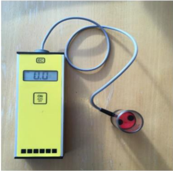
Fig. 9A: EC sensor meter for measuring nutrient solution electrical conductivity. Picture: Martin Knoop
