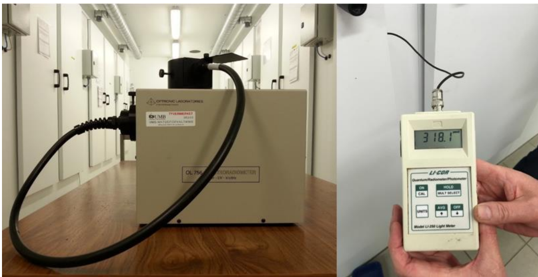
Fig 6: optronic model 756 spectroradiometer for measuring spectral composition of light and Quantum meter used in measuring light irradiance: Picture: Martin Knoop
