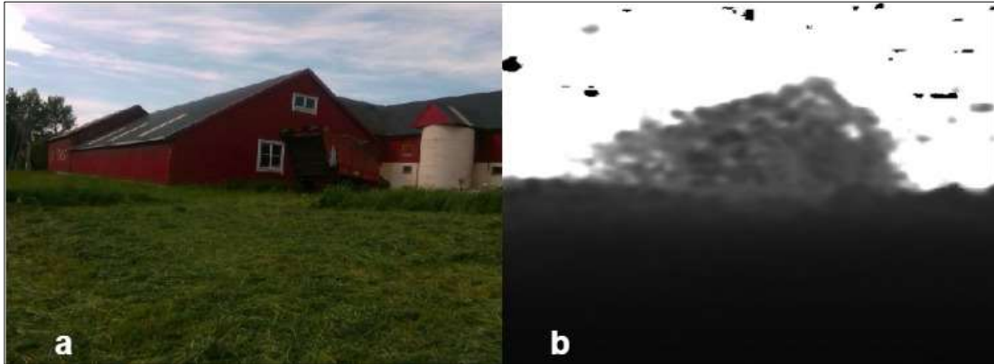
Figure 2.5: a) A coloured image showing the RGB component of the image; b) The depth component of the image produced by the RGB-D camera.
