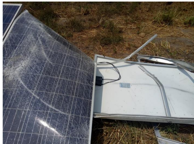
Picture 27: Hoi Nam Yen solar array after damaged by elephants
