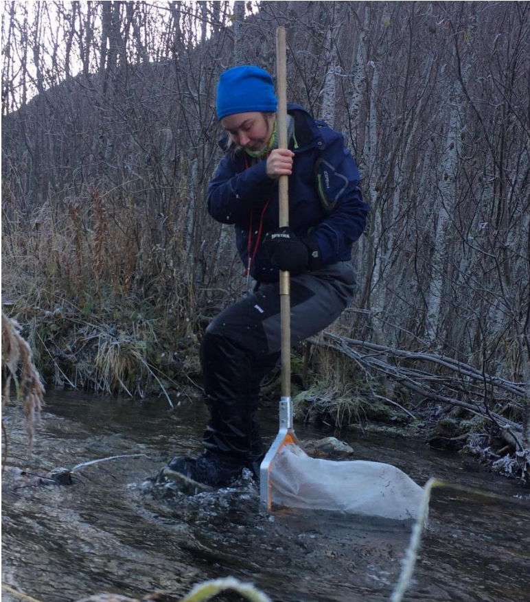
Figure 5. The net was placed into the river downstream and then kicking the bottom to collect specimens that flow into the net.
