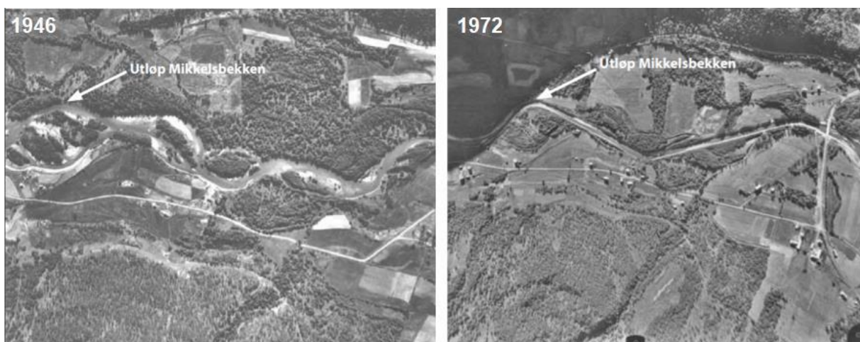
Figure 1. Changes of the shape of the river before and after the canalization of the river. In 1946, the river had a more natural shape with turns and side channels – while in 1972, the river is straightened, and the side channels are closed off as a consequence to the canalization.
