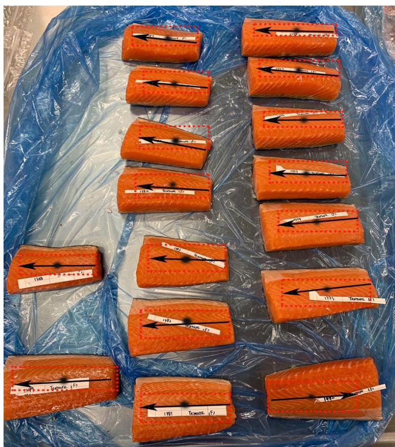
Figure 4.6, Texture measuring point marked in black dots, which were taken from middle of crossing line where muscle segments change their direction. Crossing line is designated to start from anterior dorsal fin end to fillet's another end.
