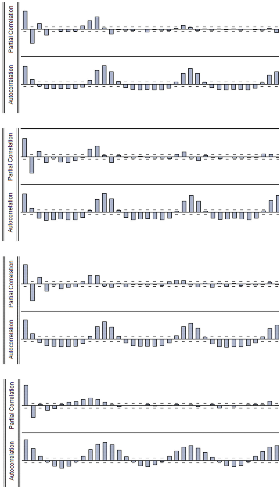
Figure 4. Autocorrelation and partial autocorrelation of standardized monthly streamflow time series for Daryan, Germezgol, Ligvan, Saeedabad stations, respectively.
