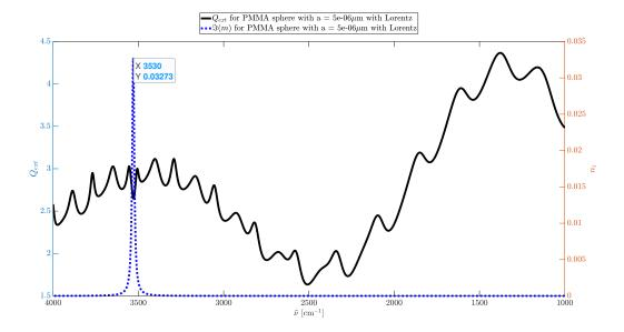
**Figure 3.42:** The  $Q_{ext}$  plotted in a solid black line versus the left y-axis for a sphere with  $n_r = 1.5$ ,  $a = 5\mu$ m and Lorentzian  $n_i$ . The  $n_i$  is given by a Lorentz function with  $\Gamma = 15 \text{ cm}^{-1}$  and  $\Lambda = 5200 \text{ cm}^{-2}$  plotted in a dotted blue line versus the right y-axis with a peak at  $\tilde{\nu} = 3530 \text{ cm}^{-1}$  with A = 0.5 as indicated by the data tip.
