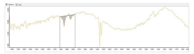
Figure 3.49: Apparent spectrum of a  $\mu$ m-sized polyethylene particle. An inverted peak is present around the high levels of scattering in the area of the  $\tilde{\nu} = 2900 \text{ cm}^{-1}$  absorption band.
