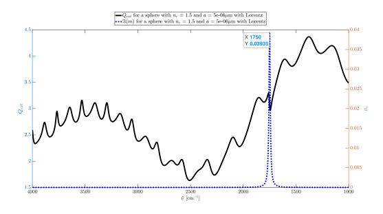
**Figure 3.46:** The  $Q_{ext}$  for a sphere with  $n_r = 1.5$  and  $a = 5\mu$ m. Lorentz peak at  $\tilde{\nu}_0 = 1750$  cm<sup>-1</sup> with A = 0.3, Lorentz FWHM  $\Gamma = 15$  cm<sup>-1</sup> and  $\Lambda = 3100$  cm<sup>-2</sup>.
