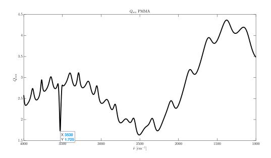
Figure 3.43: The  $Q_{sca}$  for a sphere with  $n_r = 1.5$ ,  $a = 5\mu$ m and Lorentzian  $n_i$  with  $\Gamma = 15 \text{ cm}^{-1}$ ,  $\Lambda = 5200 \text{ cm}^{-2}$ ,  $\tilde{\nu}_0 = 3530 \text{ cm}^{-1}$  and peak corresponding to A = 0.5.
