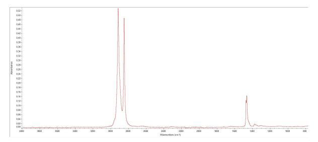
Figure 3.47: Pure absorbance (i.e. scatter-free) spectrum of a 25  $\mu$ m thick polyethylene foil.
