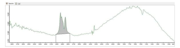
Figure 3.48: Apparent spectrum of a  $\mu$ m-sized polyethylene particle. An inverted peak is present around the high levels of scattering in the area of the  $\tilde{\nu} = 1470 \text{ cm}^{-1}$  absorption band.
