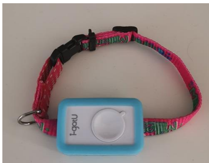
Figure 3. The GPS unit iGotU GT-120 USB Travel Logger attached to a collar. Photo: Bettina Bachmann.
