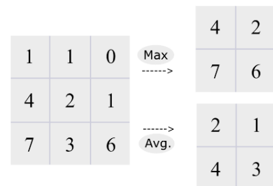
Figure 11. A simple illustration of how a picture can be processed. The grid with numbers represents a pixel with a color code. This grid is downsampled by max pooling and average pooling. Kernel = [3.2]
