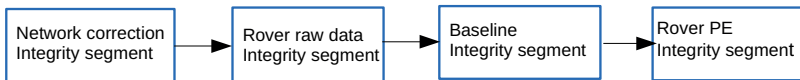
Figure 5.1: Work-flows NRTK data integrity segments for precise positioning. PE stands for position error.
