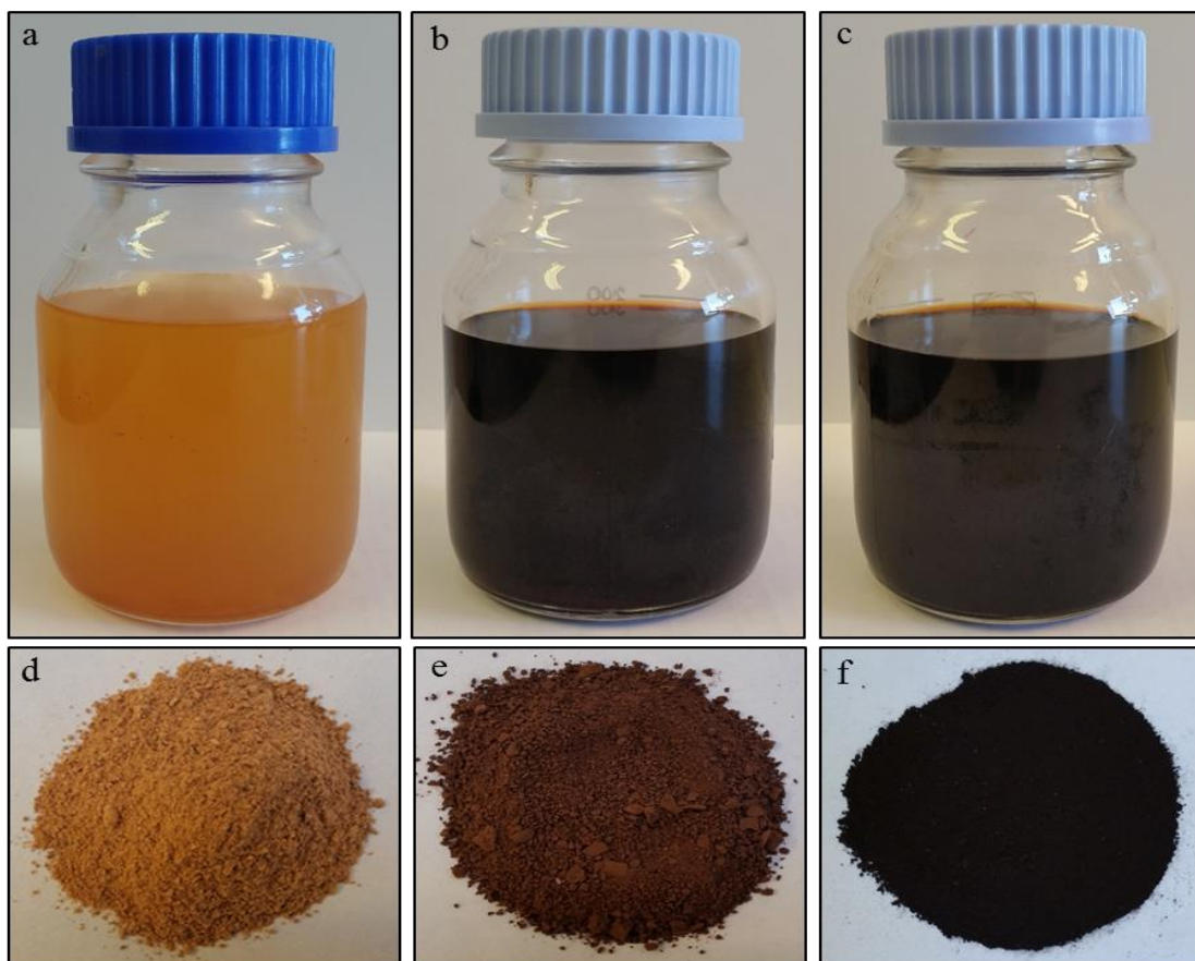
Figure 4.24: Extractable liquid (a, b, and c) and avocado seeds after the reactive extraction (d, e, and f): 75 °C (a and d), 150 °C (b and e), 225 °C (c and f).
