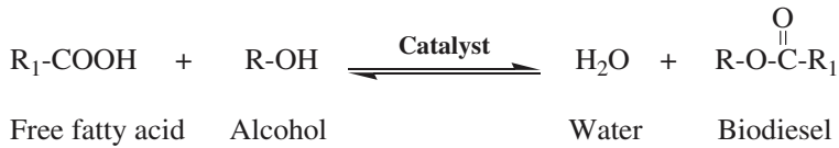
Figure 2. Esterification reaction of free fatty acid.
