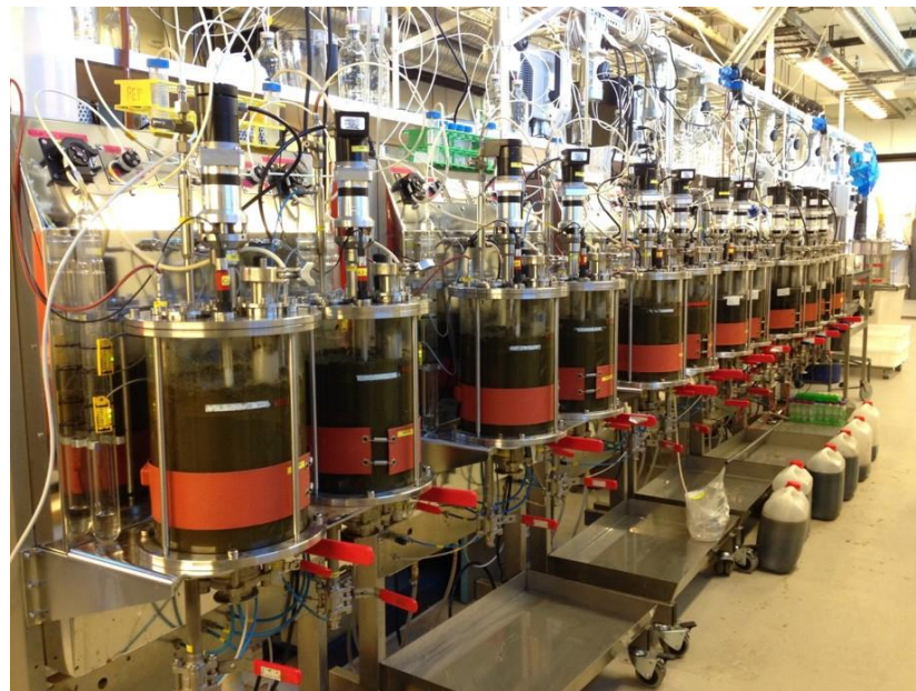
Figure 1. Laboratory-scale semi-continuously stirred tank reactors (CSTR)
