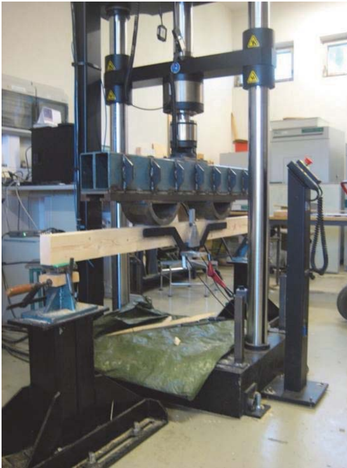
Figure 3. Four-point bending machine from Instron 5800 used for MOE and MOR testing.
