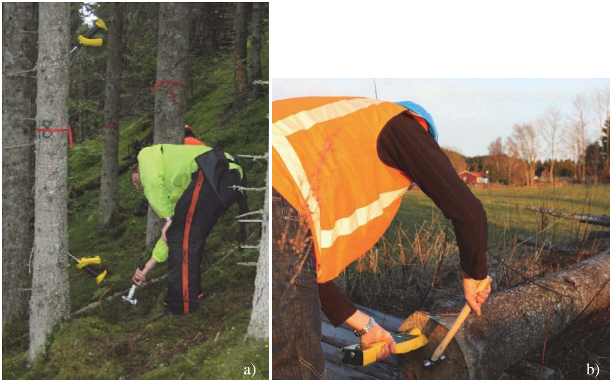
Figure 1. Acoustic measurement tools a) Hitman ST300 for standing trees and b) Hitman HM200 for logs.
