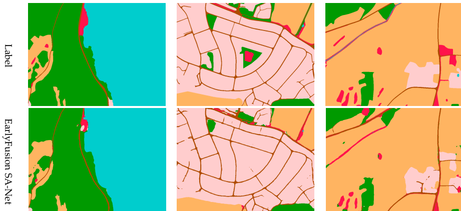
Figure 10. Final prediction results from our EarlyFusion SA-Net with RGB, HAG, and Intensity. The color legend is presented in the caption of Figure 6. The figures cover and visualize different types of areas, such as (a) forest and ocean, (b) settlement and road, and (c) cultivation and open land.
