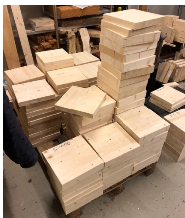
Figure 3-1 – Glulam elements picked up at Moelven Limtre AS, ready for specimen production.
