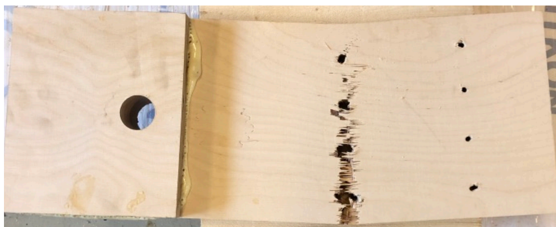
Figure 5-5 – Fracture appearance of the plywood plate in test group U-1-0D.
