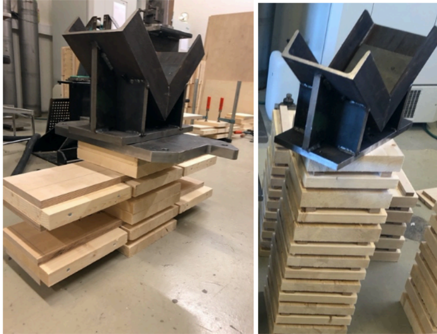
Figure 3-4 – Loading of glued parts for the curing process. Heavy steel objects were used to gain sufficient curing pressure.
