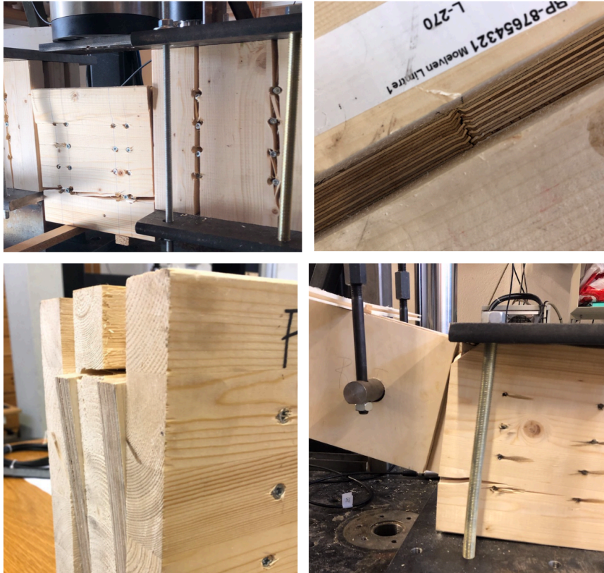
Figure 3-2 – Complications experienced in the preliminary testing. The top row presents issues from the symmetrical tests (splitting and collision of plywood plates) and the bottom row from the unsymmetrical tests (splitting and collision between plywood and steel plate).
