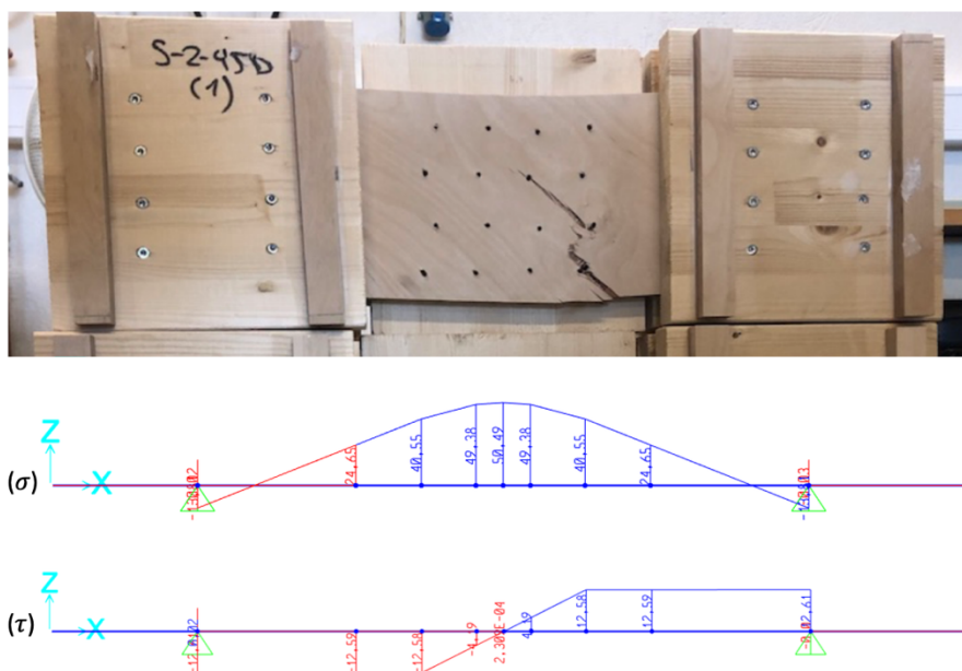
Figure 4-13 – Comparison of fracture location in S-2-45D and tensile/compressive ( \sigma ) and shear ( \tau ) stress distribution from SAP2000. The values displayed are measured in MPa.
