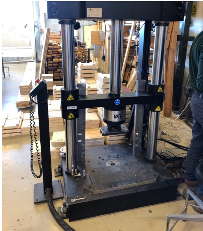
Figure 3-16 – INSTRON hydraulic press machine used in the experimental testing.
