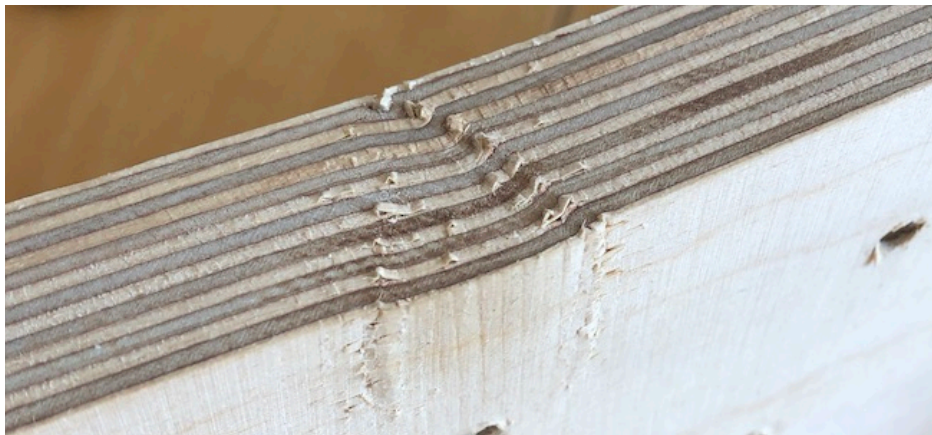
Figure 5-1 – Compressive failure of the plywood as a result of bending of the plate.
