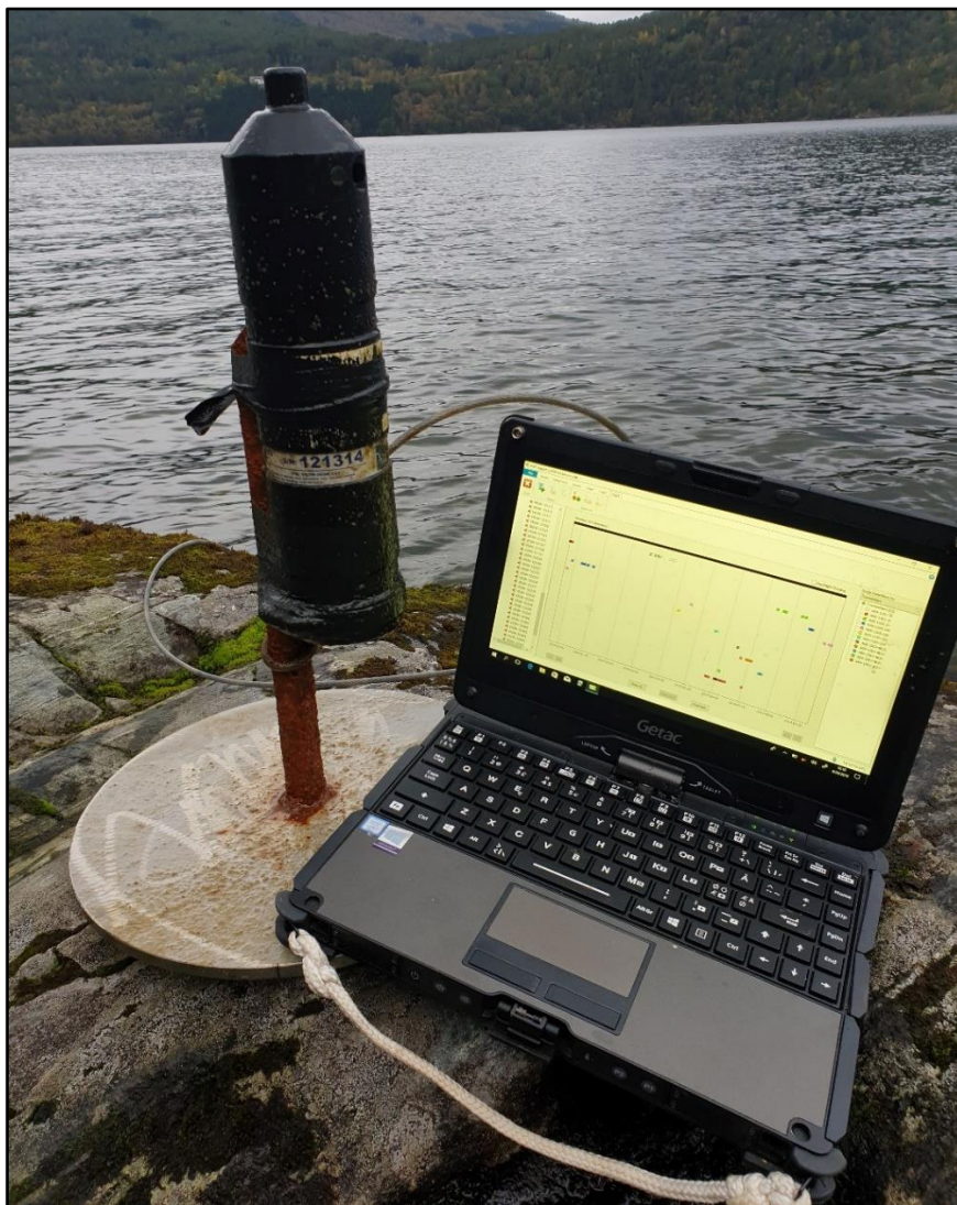
Figure 3: Here we see a picture of an acoustic receiver (VR2W, Vemco, Canada) strapped to a metal parabola that keeps the receiver in place in Hornindalsvatnet. We can also see the mooring wire attached to the metal parabola, and the transferring of observations stored on the receiver via Bluetooth to a laptop. When the transferring was complete, the receiver was put back in the lake. Photo: Aksel Fiske.
