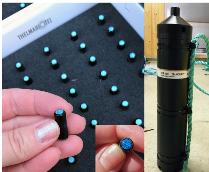
Figure 2.5: Tags with ID numbers to the left, and the TBR 700 receiver to the right.
