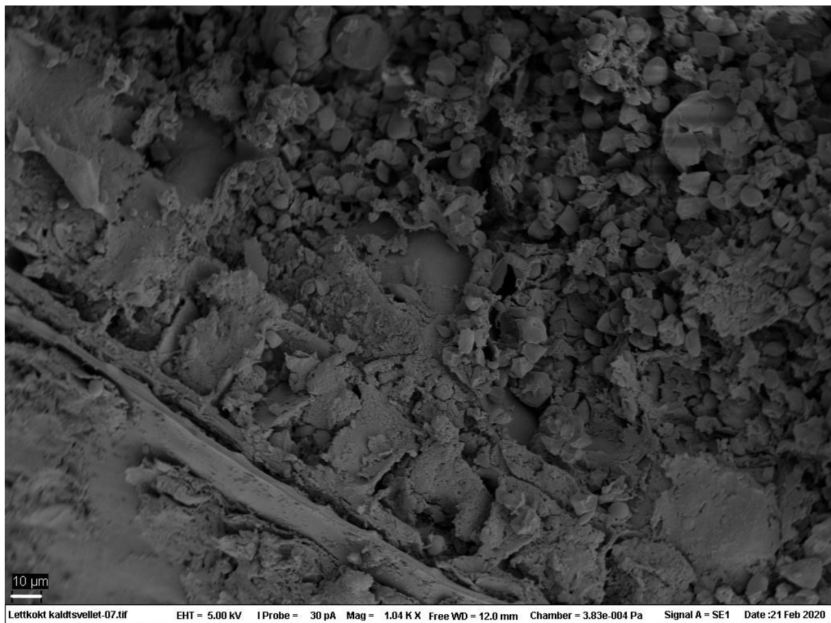
Figure 5.8: Micrograph of a cold swollen fast cooking oat flake from the SEM.
