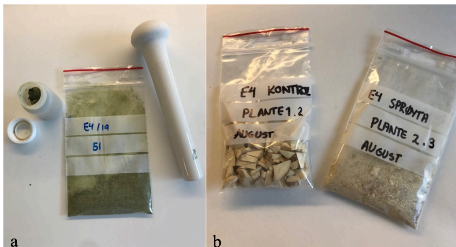
Figure 4.8: Sample preparation and homogenization: a) freeze dried leaves from a plastic vial transferred to a plastic bag and crushed with a mortar, b) freeze dried potato core before and after crushing.
