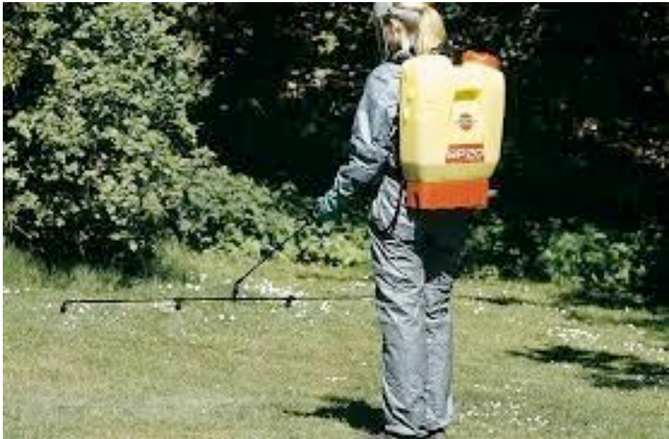
Figure E.1: Illustration of a Hardi BP 20 back pack sprayer with a boom of 4 nozzles (last nozzle behind the legs on the woman in the photograph) (Agronom, 2015).
