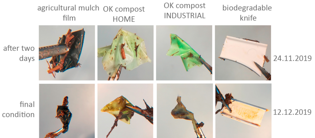
Figure A4: Visual examination of the 1.5L incubation at 35°C. None of the biodegradable plastics have started fragmenting or degrading in the period of 20 days.
