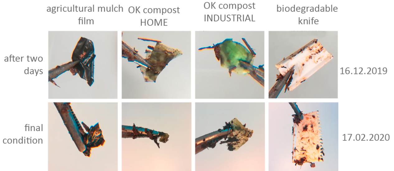
Figure A3: Visual examination of the 1.5L incubation at room temperature. Though the OK compost HOME sample started fragmenting after 116 days of incubation, the other plastics remained intact. It should be noticed that these samples had been examined oftentimes over the course of several months which added a certain physical stress.
