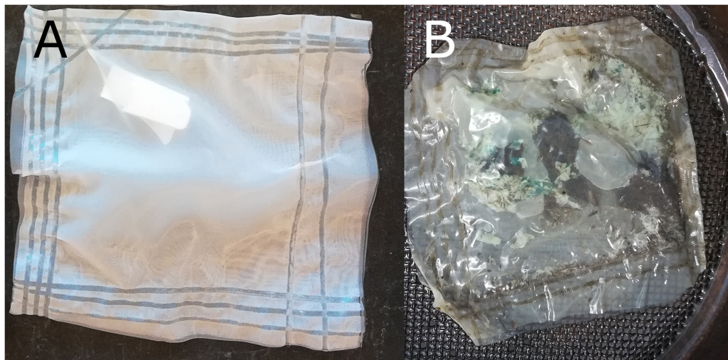
Figure 3: Examples of nylon bags before (A) and after (B) incubation. Fragmentation of the biodegradable plastic in picture B can be seen. A shows the seams used for identification of the bags.
