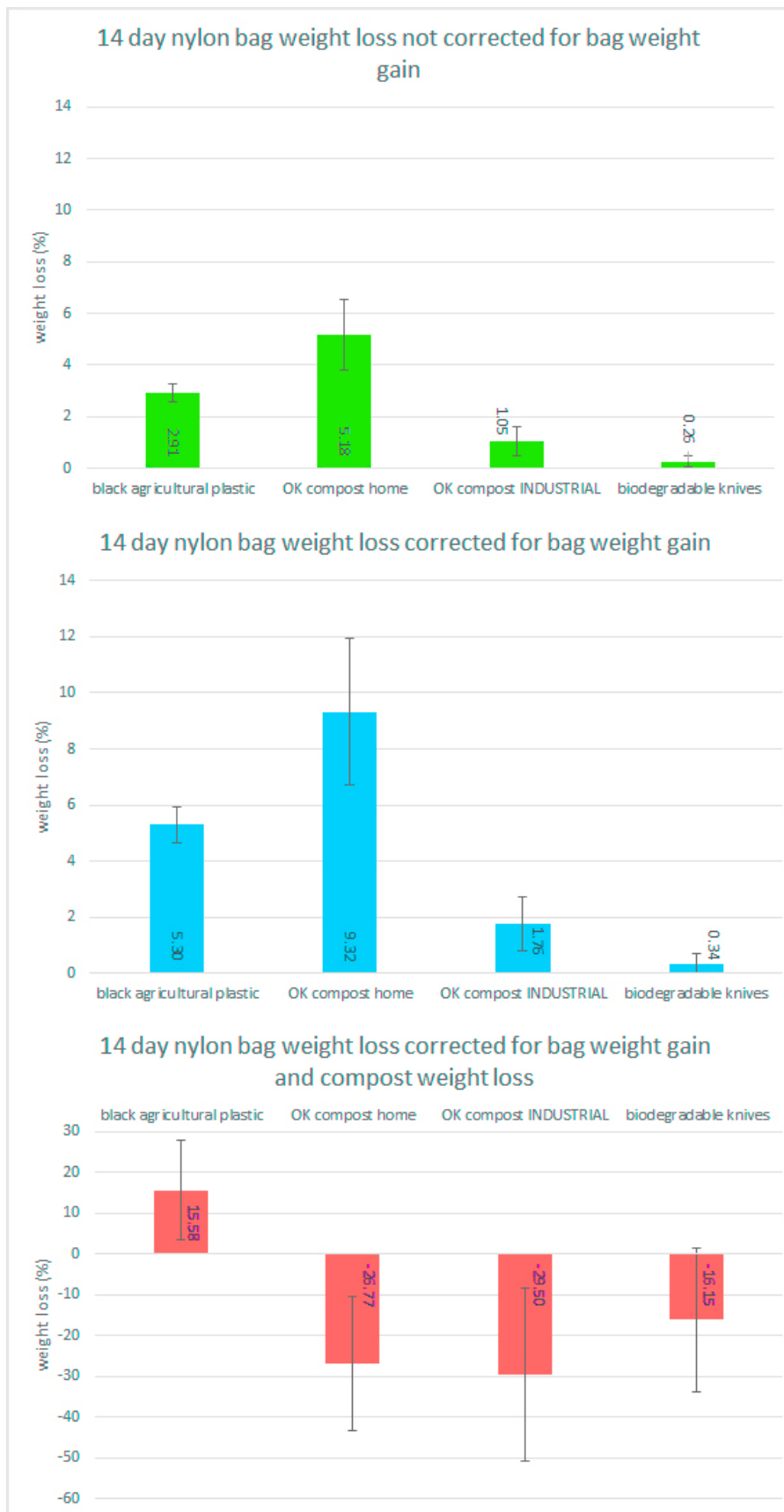
Figure 10: Weight loss of the four biodegradable plastics inside of the 50µm mesh size nylon bags after 14 days incubation. Empty bags used for nylon bag weight change correction had n=5 with an average weight change of -0.2% and a standard deviation of 0.5. The compost used for weight change correction had n=5 with an average weight change of -30.8% and a standard deviation of 3.1. Raw data can be seen in Table A5.
