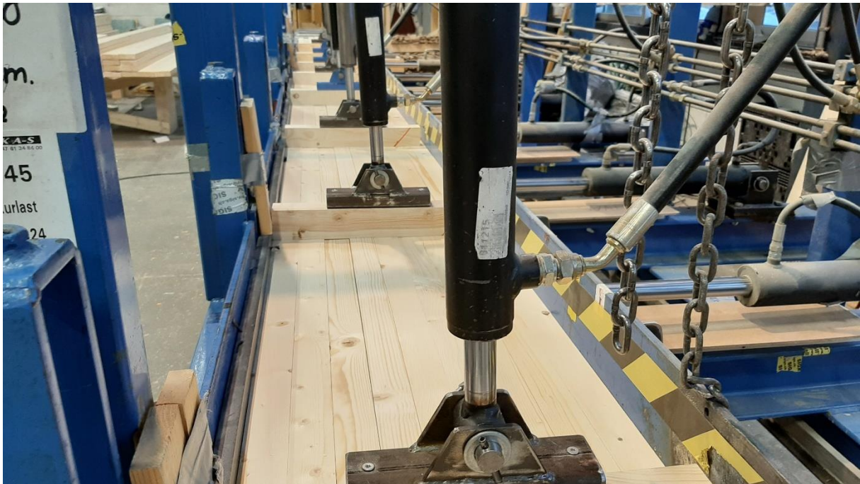
Figur 3.2-5 - Presset element i jiggen.
