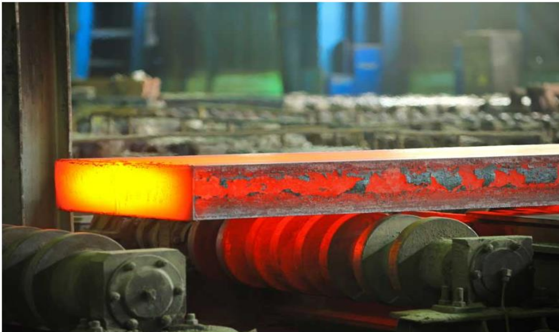
Figure 8 Hot rolled steel
