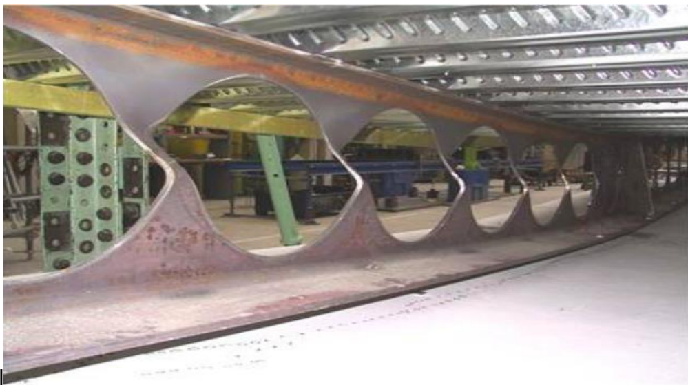
Figure 19 Web-post buckling mode
