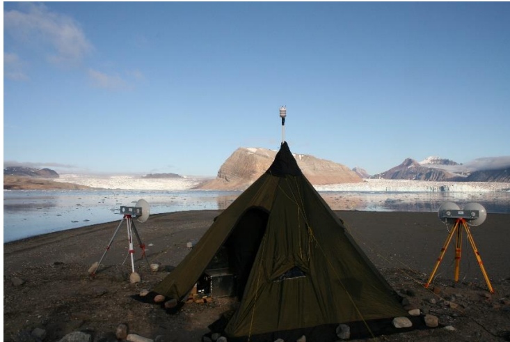
Figure 13. Picture from the 2008 measurements of Kronebreen from Pynten. To the left is the transmitting antenna and to the right are the two receiving antennas forming the interferometer. Photograph courtesy of ISPAS AS.
