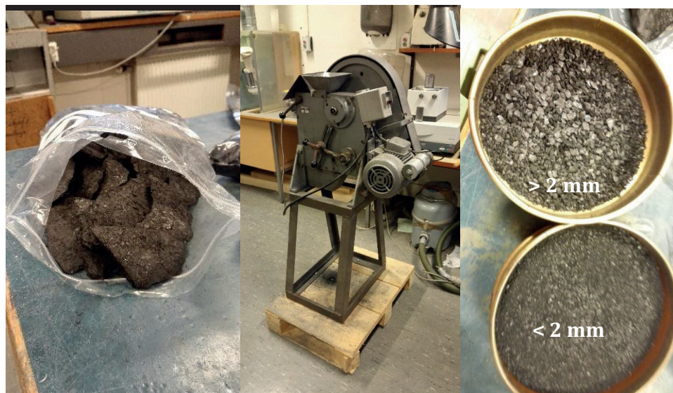
Figure 10: Alum shale used for the experiments (before crushing, left), jaw crusher for crushing of alum shale debris (middle) and sieving of alum shale through 2 mm (right).
