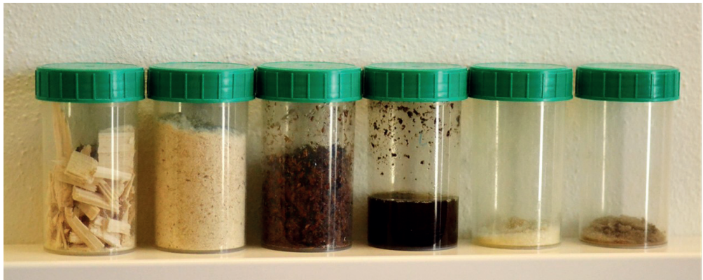
Figure 5. Samples taken at each step in the Norway spruce GGM production process. Left to right: dry wood chips, chips milled to <2mm size, steam explosion slurry, liquid fraction of the slurry recovered with the cider press, dried retentate from the 5 kDa cutoff, dried permeate of the 5 kDa filtration.
