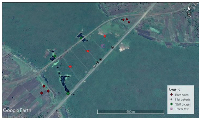
Figure 3b: The instrumentation site along Naigombwa River, bright red points represent locations of automatic water divers
