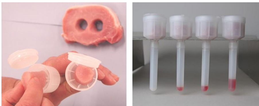
Figure 7. Set-up for EZ-DripLoss measurement showing sampling of cylindrical meat pieces and the storage containers for meat samples. Photo: Danish Meat Research Institute.
